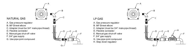
The gas pressure regulator must be installed in the gas line – failure to install a pressure regulator will void the equipment warranty. The regulators supplied with ranges have 3/4" NPT connections; the regulator is adjusted at the factory for 5" W.C. (water column) manifold gas pressure (natural gas) or 10" W.C. manifold gas pressure for propane gas operation.
