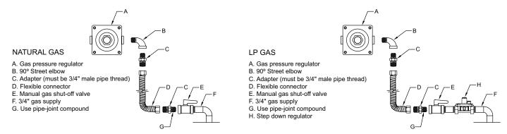
The gas pressure regulator must be installed in the gas line – failure to install a pressure regulator will void the equipment warranty. The regulators supplied with Radiant Broilers have 3/4" NPT connections; the regulator is adjusted at the factory for 5" W.C. (water column) manifold gas pressure (natural gas) or 10" W.C. manifold gas pressure for propane gas operation.
